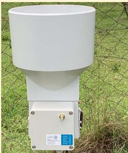
Automatic Rain Gauge installed at Ruiru Dam. The instrument measures, monitors, record and transmit rainfall data to a base station.
